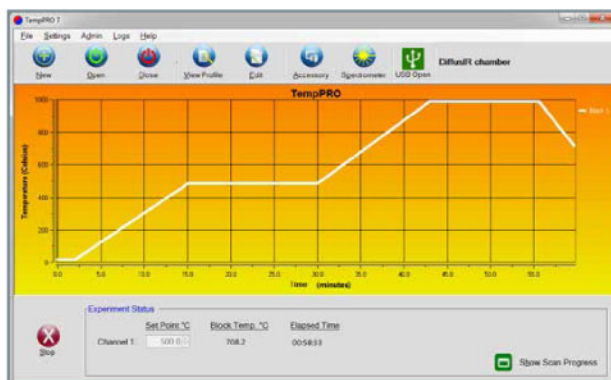
PIKE TempPRO software provides a graphical interface for temperature control and kinetic measurements.
