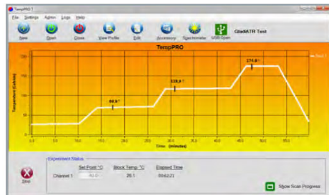
PIKE TempPRO™ software for graphical setup and automated data collection for thermal experiments.
